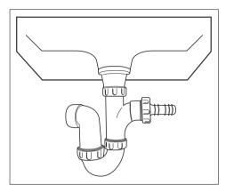
Push the drain hose onto the spigot and secure with a clip, ensure a loop is formed in the drain hose (see diagram) to prevent waste from the sink entering the appliance. If you intend to drain the hose from the machine into a sink, make sure that the sink is empty and the plug hole is not blocked. Use the plastic "U - Piece" supplied.
